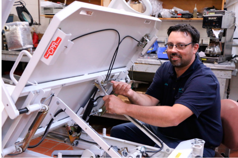
Meet member James Young, of Local 119. James is an Equipment Repair Technician at the Victoria General. He's currently working on a hospital bed, testing the CPR release button, the bed scales, and making sure that all the motors are functioning correctly.
